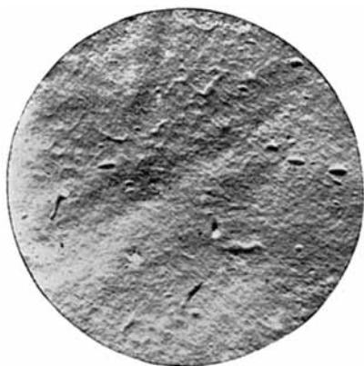
Fig. 6. Impressions of small particles on the surface of a swollen pine sulfate fiber fragment. \times 5000 .
