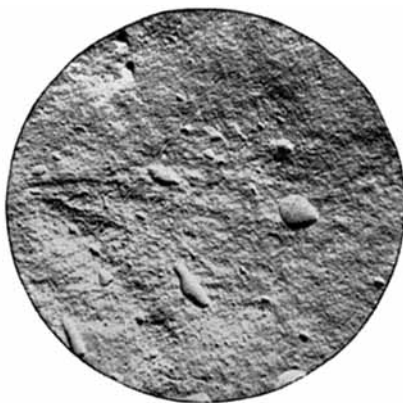
Fig. 6. Impressions of small particles on the surface of a swollen pine sulfate fiber fragment. \times 5000 .
