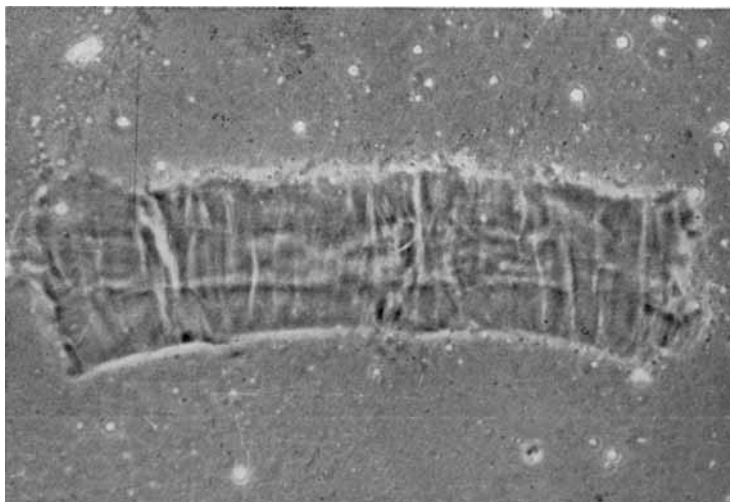
Fig. 1. A typical swollen fiber fragment in viscose solution as seen under the phase microscope. Particles surrounding the fragment belong to the group of the "granular dispersion." \times 200 .
